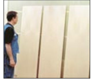
4 Checking and sorting panels according to colour and grain pattern.
